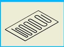
2. Apply adhesive to the back side of the end skin staying about an inch from edges.
