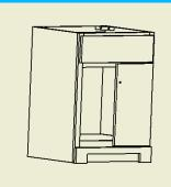
1. Remove the door or drawer on the side that the end skin is to be applied.
